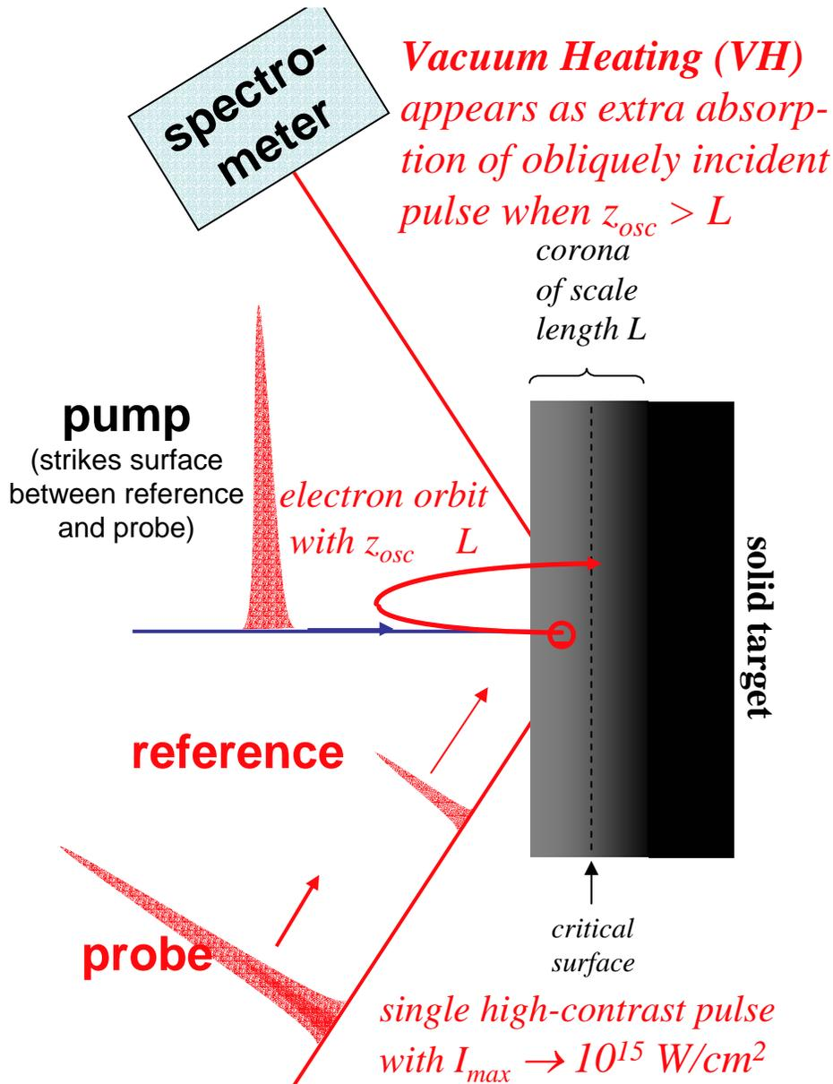
$\tau_p = 100 \text{ fs}$ ,  $\lambda = 620 \text{ nm}$ ,  $I_{\text{pump}} \approx 10^{15} \text{ W/cm}^2$ ,  $\theta_{\text{probe}} = 60^\circ$
