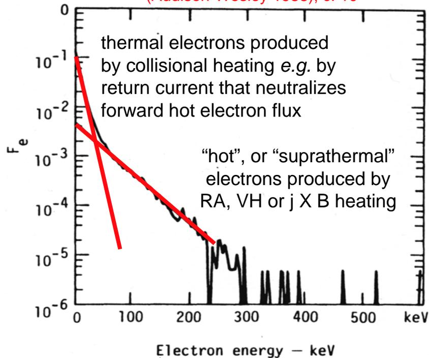
Measured hot electron energy distribution from 50  $\mu\text{m}$
