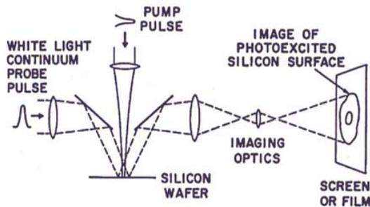
MAJOR EVENTS:  $\left\{ \begin{array}{l} \Delta t < 0: \text{ semiconducting Si surface } (R = 0.3) \\ -0.04 < \Delta t < 0.04 \text{ ps: pump absorbed} \\ \Delta t \approx 1 \text{ ps: liquid metal Si surface } (R = 0.6) \\ \Delta t \geq 10 \text{ ps: absorption from ejecta } (R \rightarrow 0) \end{array} \right.$
