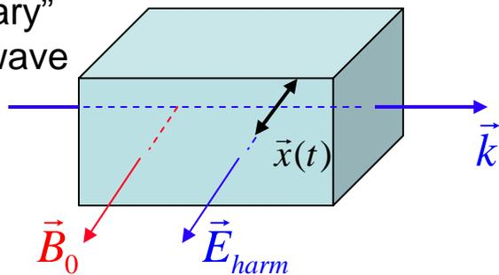
$$\vec{x} \times \vec{B}_0 = 0 \quad \Rightarrow \quad \vec{P} = -\frac{n_e e^2}{m\omega^2} \vec{E}_{harm} = -\epsilon_0 \omega_p^2 \vec{E}_{harm}$$
