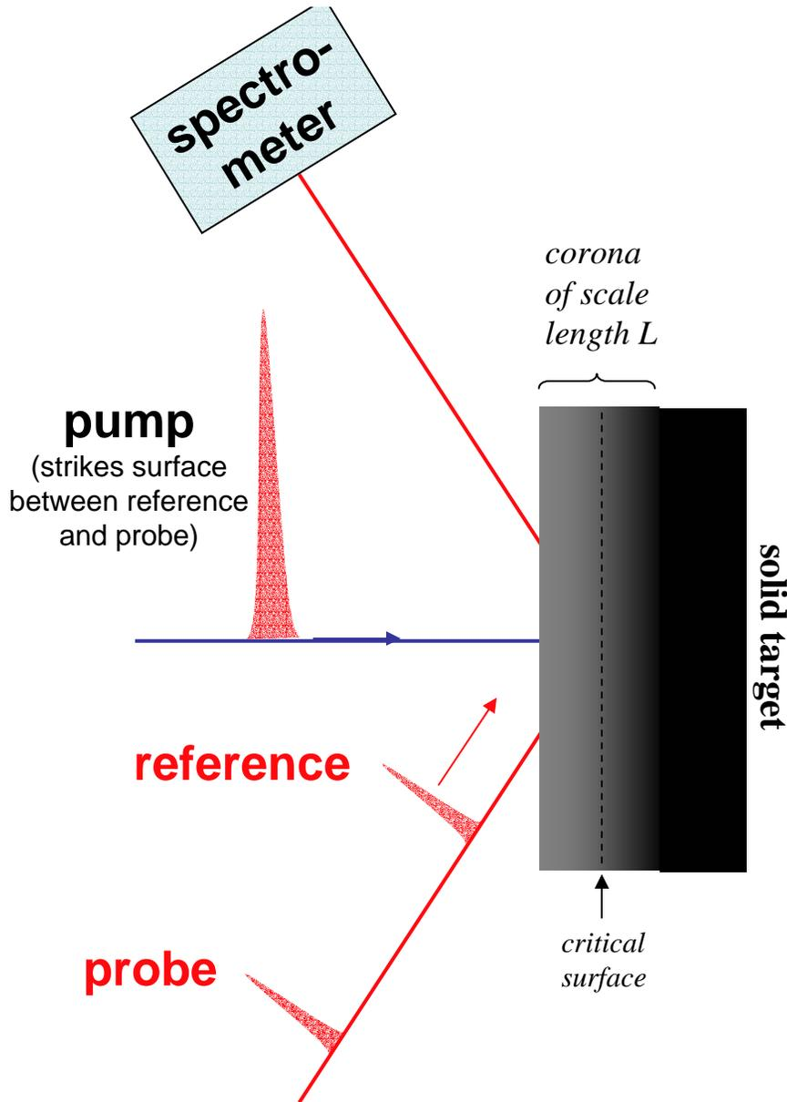
$$\tau_p = 100 \text{ fs}, \lambda = 620 \text{ nm}, I_{\text{pump}} \approx 10^{15} \text{ W/cm}^2, \theta_{\text{probe}} = 60^\circ$$
